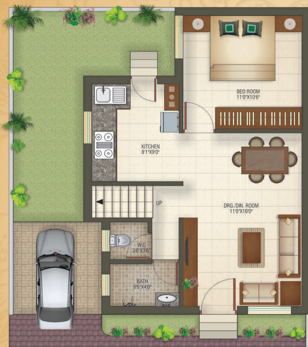
GROUND FLOOR PLAN S.B.A : 663.00 SQ.FTS. Stair Cabin : 86.00 SQ.FTS.
